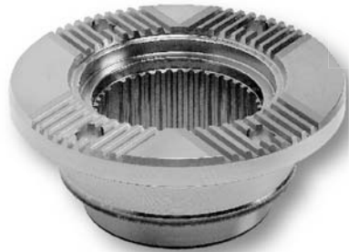
Design according to DIN ISO 8667 – Induction-hardened and lead-free ground seal bearing surface – Internal splines – Cross-serration 70°
