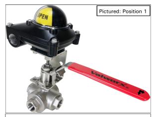
\*Note: Installer can easily change flow path for 3-way T-Port from standard shipped position to an alternate Position 1 with limit switch indicating "Open" in the field as required. Position 1 options are shown below. User may remove valve portion only and rotate top male valve stem to desired Position 1. A 90° turn to will result in corresponding Position 2, with limit switch "Closed". Flow path on handle may no longer match.
