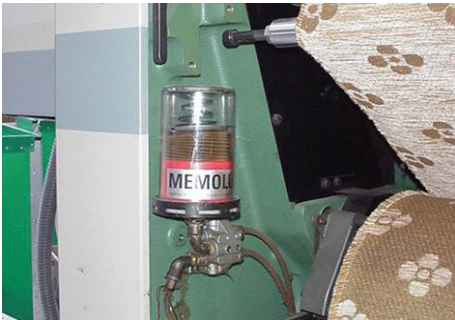
Textile industry: Picanol weaving loom bearings.
