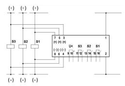
The figure represents the connections of a VDB30 OP that supervises alternatively three trip coils
